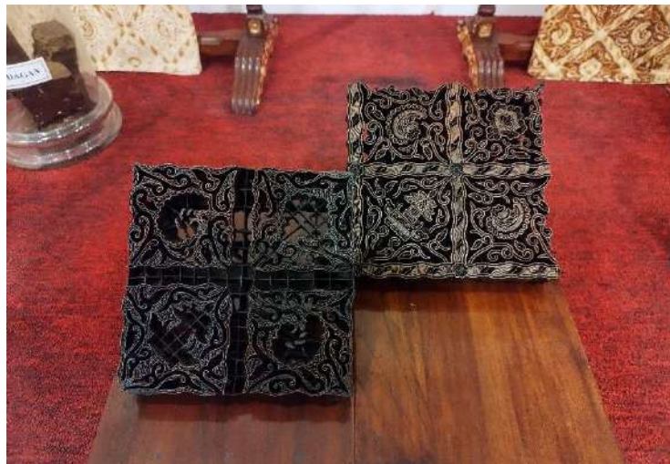
Figure 6. Batik Sidomukti stamping tool
